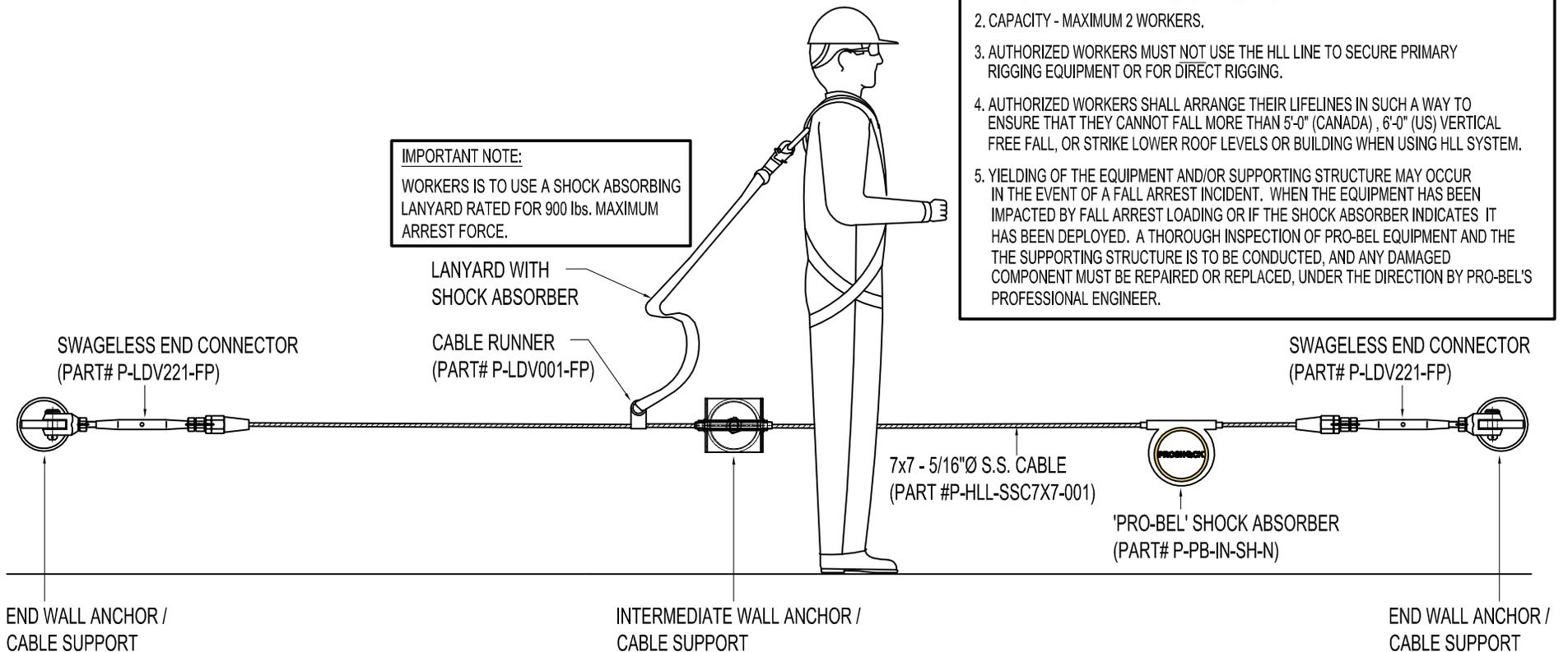
**HORIZONTAL LIFELINE FALL ARREST SYSTEM ASSEMBLY - HANDS FREE SYSTEM - PRO-SHOCK**
