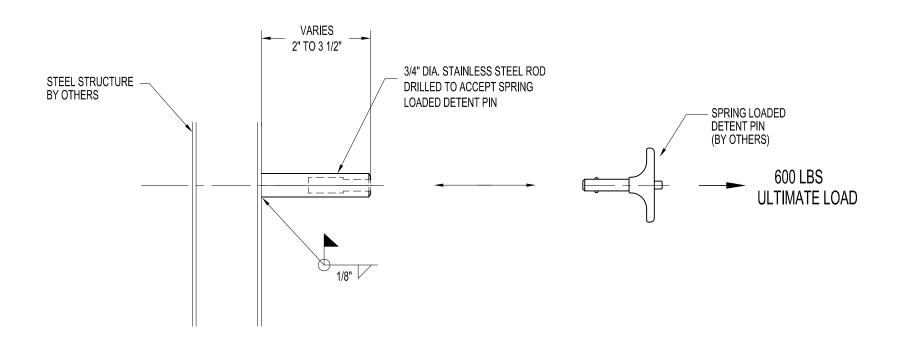
A-STB-RD1512: WELD TO STRUCTURE STABILIZATION TO SUIT SPRING LOADED DETENT PIN
