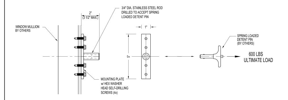
A-STB-RDP112A1-02: BOLT TO MULLION STABILIZATION TO SUIT SPRING LOADED DETENT PIN
