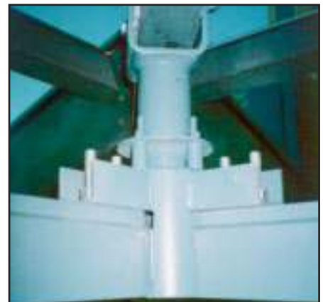
Monorail corner-turning hub secured to steel rafter provides automatic turning at corners. See worms-eye view on page M-9.
