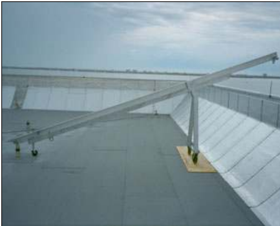
This Pro-Bel portable long reach outrigger beam system was designed to clear a high parapet wall and features a light weight reinforced aluminum beam with dolly wheels for ease of movement. Outrigger materials i.e. aluminum, stainless steel, rubber wheels, etc. withstand year-round exposure when stored on the roof. HealthSouth Corporation, Melbourne, Florida.
