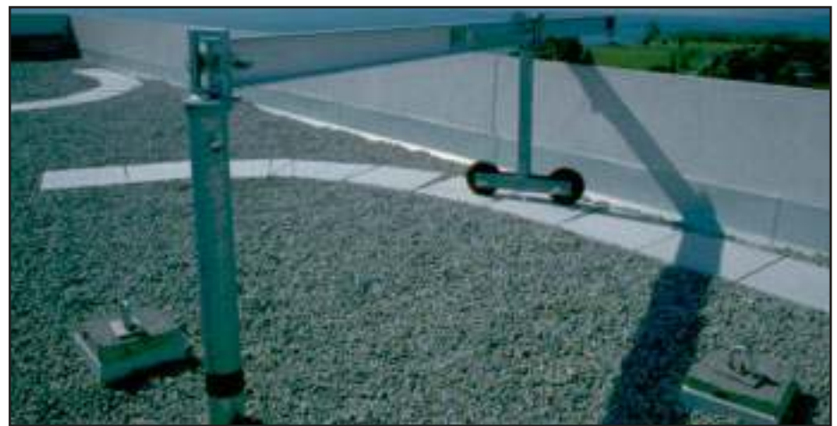
Pro-Bel portable swivel-type outrigger beam with dolly wheels. Pavers are recommended to facilitate wheel movement and protect roof from loading on front dolly wheels. Note pier mounted independent lifeline U-bar anchors in field of roof.
