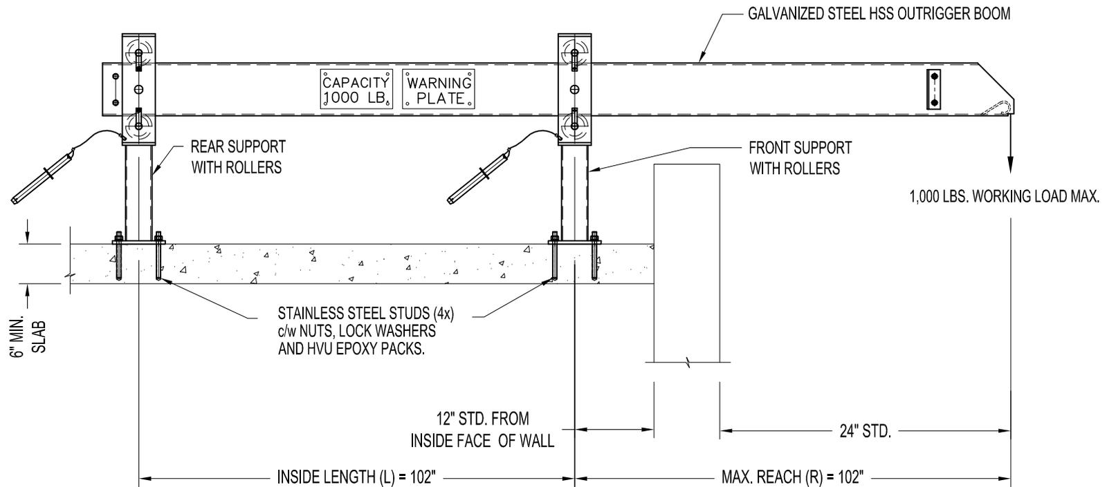
**A-OR-7740-102: FIXED OUTRIGGER ASSEMBLY (UP TO 8'-6 REACH) - ADHESIVE**
