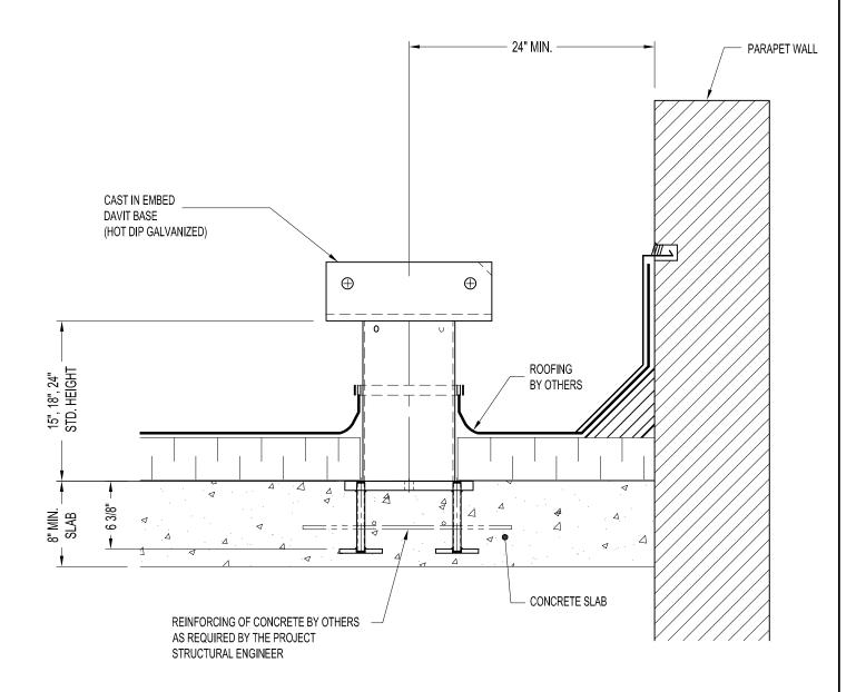
DB2-23108: 200 SERIES DAVIT BASE ASSEMBLY (ONE PIECE CAST IN EMBED) - w/ NO U-BAR
