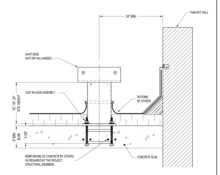
DB2-23103: 200 SERIES DAVIT BASE ASSEMBLY (CAST IN CAGE) - WITHOUT U-BAR
