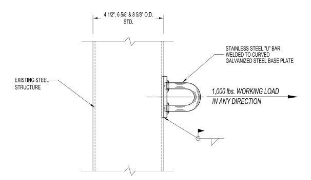
PB80SC: WELD TO ROUND STEEL STRUCTURE WALL ANCHOR
