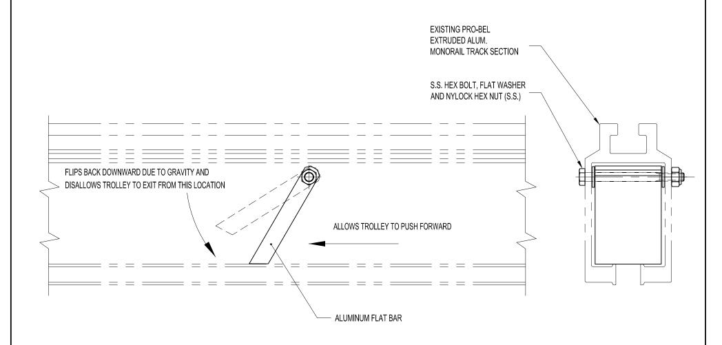
MNES40: PRO-BEL MONORAIL TRACK SECTION GRAVITY LOCK (END STOP)
