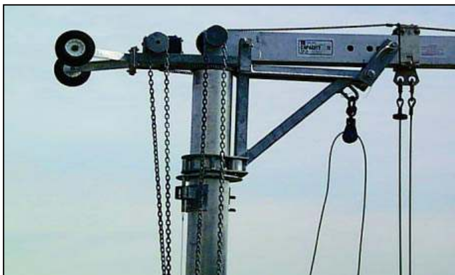
Close-up photo showing top of Pro-Bel Tall Davit. Equipped with two gear chains - one to facilitate davit arm rotation and one to facilitate movement of rolling trolley inboard or outboard under load.
