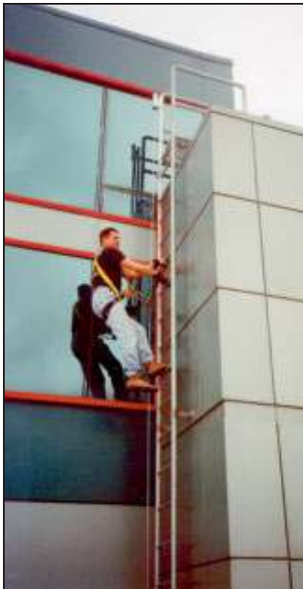
Worker is connected to continuous, tensioned vertical steel cable on this fixed Pro-Bel ladder. In the event of a slip or fall, the connector locks onto the cable within inches of a fall.
