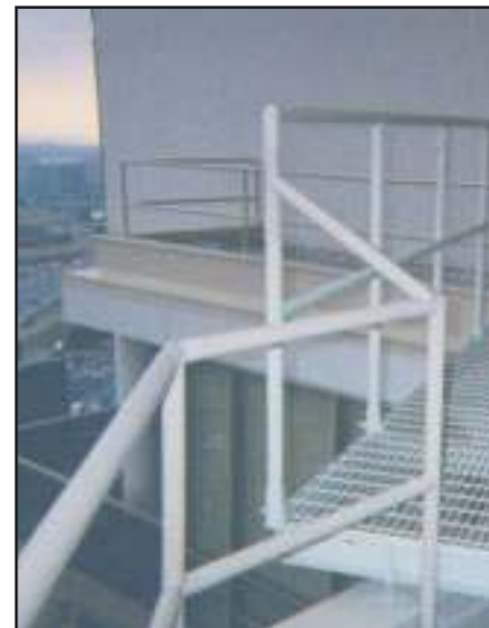
Pro-Bel standard 42" (1067 mm) high tubular aluminum safety guardrail for edges having a drop greater than 4'-0" (1220 mm).
