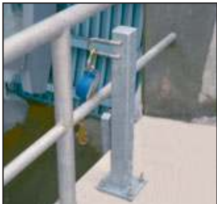
One of many Pro-Bel safety anchor retrofit products. U-bar is welded to steel post which is affixed to concrete walkway using epoxy adhesive anchor bolts. Retractable lanyard is attached to U-bar. Also see safety guardrails data on page I-7.
