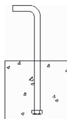
SECTION DETAIL EXAMPLE ROPE GUIDE/ LINE STOP (SURFACE MOUNTED TYPE SHOWN IN PHOTO BELOW)
