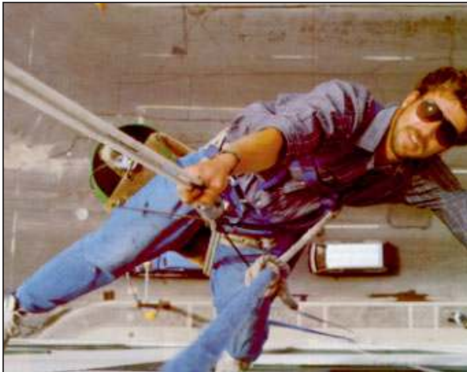
Bosun's chair is the equipment of choice among window cleaners. Pro-Bel safety anchors provide a practical means for securing lifelines or suspension equipment such as a bosun's chair with descent control.
