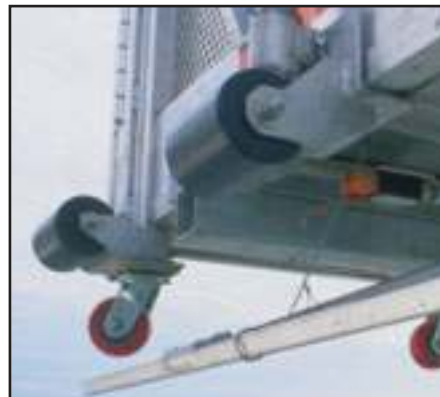
Photo above shows non-marking building face rollers. Many permanent platforms require extendable building face rollers (See photo at top of page P-4).
