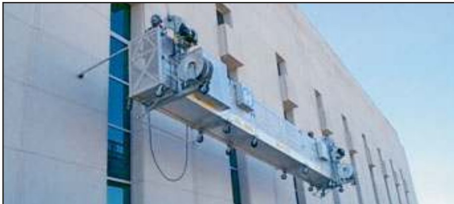
Photo shows how face roller extensions are used to clear window canopies as well as roof mounted light standards located on a lower roof.
