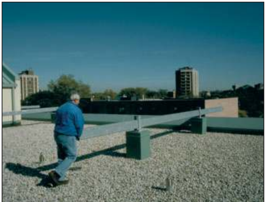
Pro-Bel fixed outrigger beam systems are designed to remain in place. Sliding beam, as shown above is ideal where inboard roof space is not restricted. Sliding beams typically span over 10'-0" (3 m) beyond the fulcrum and are available in aluminum or steel.
