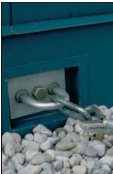
Above are examples of typical Pro-Bel wall anchor (left) and roof anchor (right) which can be used for both the securement of lifelines and for the tie-back of suspension equipment e.g. conventional outriggers and parapet wall clamps, or for the direct securement of a bosun's chair (direct rigging).
