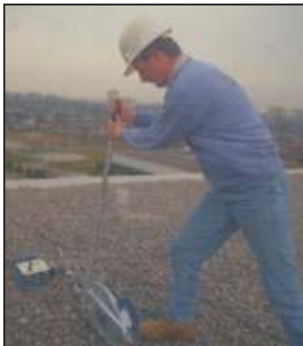
Load tester being used to verify strength of Pro-Bel roof anchor. Opposite end of cable is secured to wall anchor or other suitable structure.
