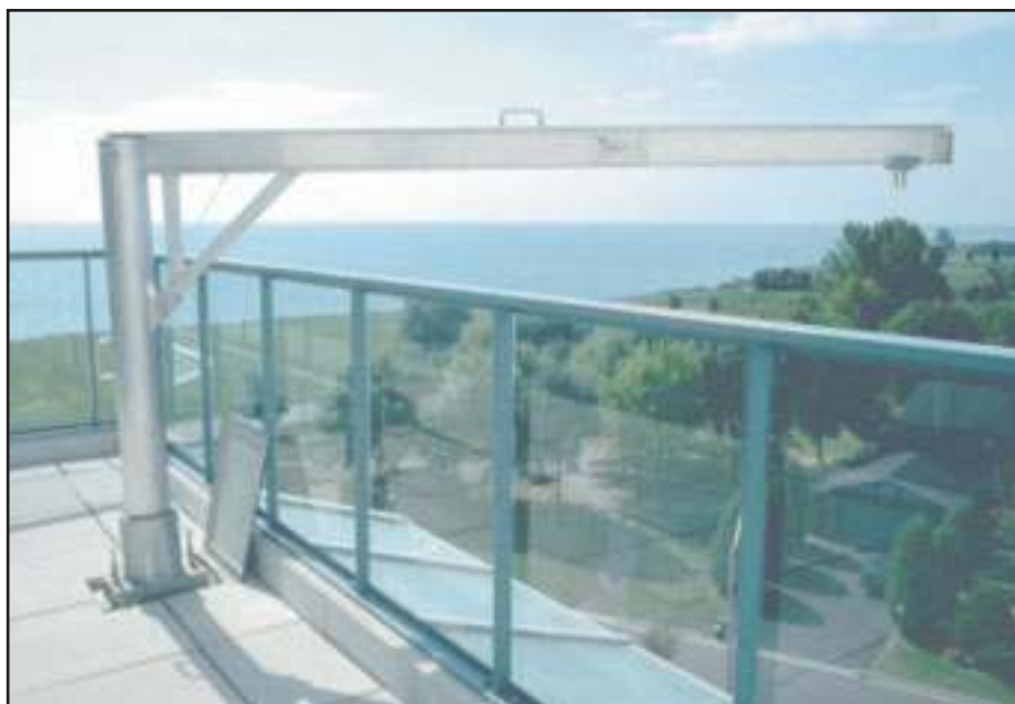
Pro-Bel portable, ground rigged davit assembly with recessed base is typically used where a flush mounted deck appearance is required or desirable between maintenance operations. Note deck cover plate leaning against rail.
